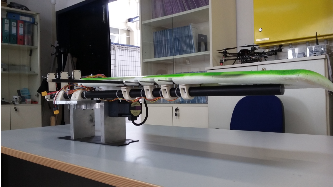
Figure 6.8: Protruding calibrator geometry under the wing
