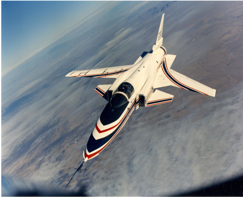
Figure 3.5: An airdata boom mounted on the nose of an experimental aircraft
