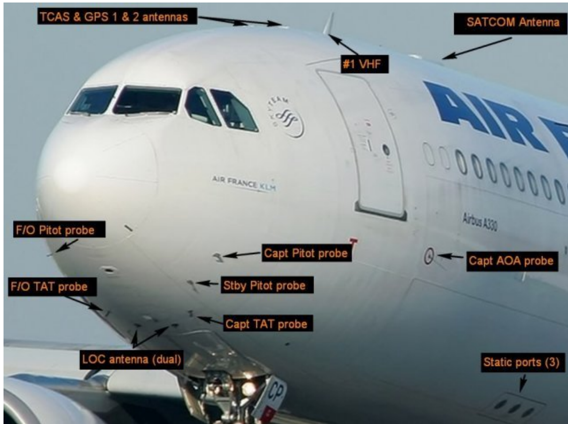
Figure 3.4: Multiple and redundant air data instruments on a passenger jet
