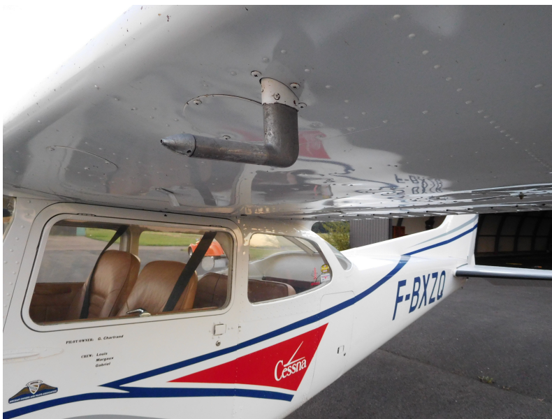
Figure 3.6: A Pitot probe on a personal aircraft
