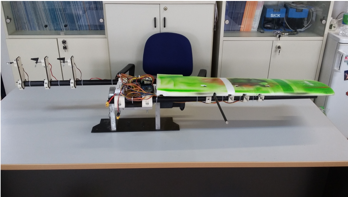
Figure 6.7: The calibrator with the wing installed
