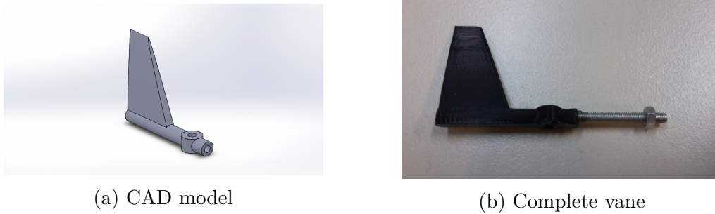
Figure 5.3: The custom-made wind vane
