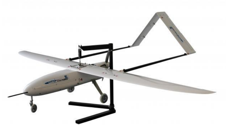
Figure 3.8: A UAV equipped with a Pitot-static probe
