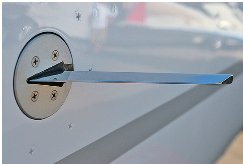
Figure 3.3: An angle-of-attack sensor installed on a passenger airplane
