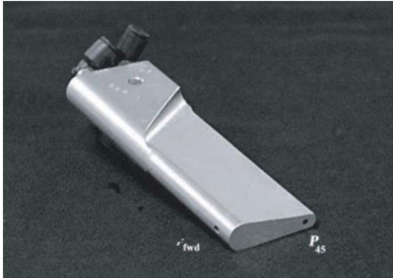
Figure 3.7: The two-port sensor from [12]
